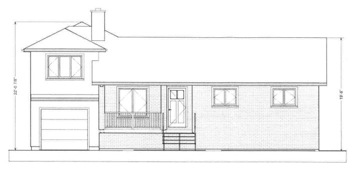
ELEVATION A SCALE 1/8"=1'-0"
